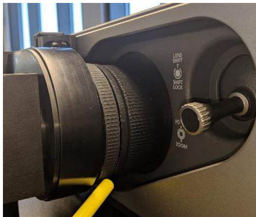
Figure 56 – Focus dial on projector
