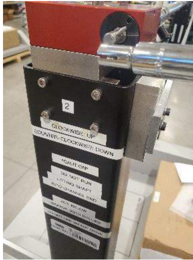
Figure 17 – Gear box and keyed-socket bit
