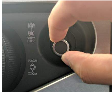
Figure 50 - Image alignment joystick on projector
