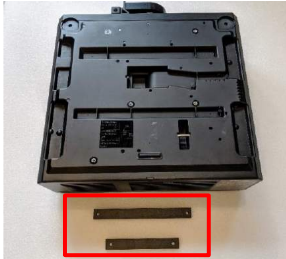
Figure 38 Projector upside down on foam for preparation
