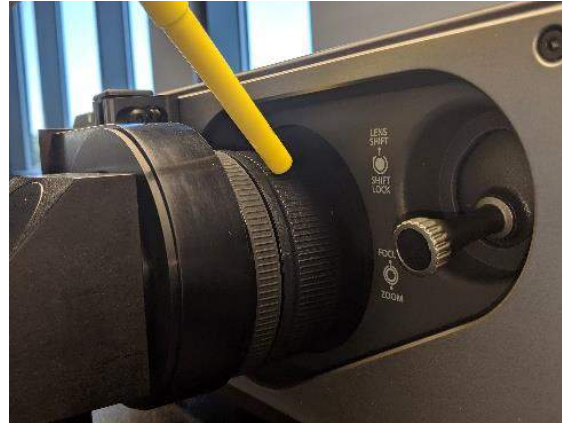
Figure 53 - Zoom dial location on projector
