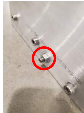
Figure 31 - Side rail lock nut
