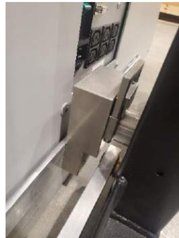
Figure 13- Lock the gate on the bushing
