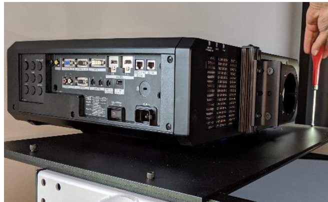
Figure 44 - Securing projector assembly to mounting rails
