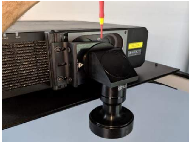
Figure 46 - Fisheye lens set screw location
