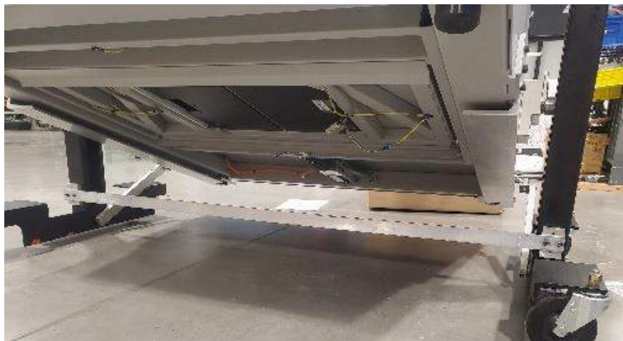
Figure 18 – Stabilizer Bar connected to bottom of dollies
