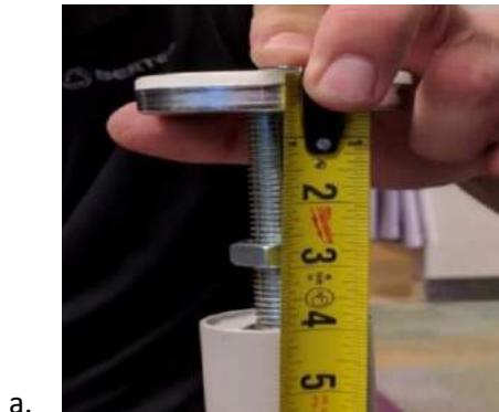
Figure 32 - Measuring mount feet are screwed into the legs
