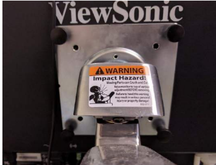
Figure 57 - Touchscreen monitor attaches with the outermost set of 4 screw holes
