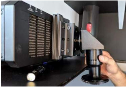
Figure 45 - Connecting fisheye lens to projector
