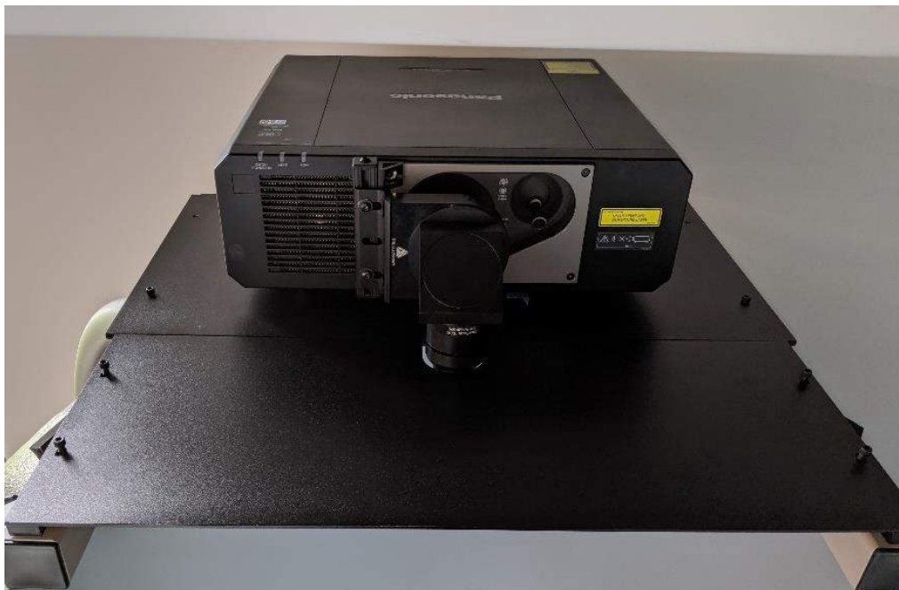
Figure 48 - Position of Projector Lens Cover Plate
