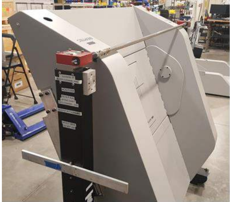
Figure 24 – Raised to max just before drive shaft interferes with base
